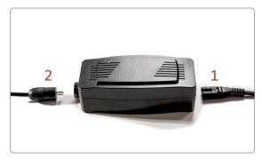
Connect the power cable [1] with the transformer and then with the socket. Plug the cable coming from the sofa into the transformator [2]. By slightly touching the TOUCH-sensor in the front the function extends smoothly. By slightly touching the TOUCH-sensor in the back the function retracts. Some models with double motor have 4 TOUCH-sensors. Two at the front for moving the seat or the footrest, two in the back for moving the backrest.
